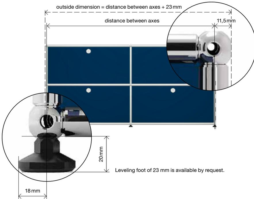
The USM Haller system provides a wide variety of elements in standard sizes. Heights, widths and depths are indicated as shown below. All measurements in mm refer to the distance between axes.
