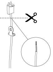
2. Unfasten grub screw at the cable grip to release cable.
