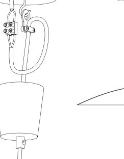
5. Control cable's length by unscrewing the cable grip screw and sliding the cable through. Restore power at the fuse box. Your product is now ready to use.
