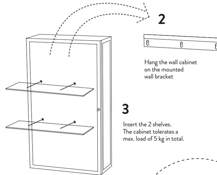
Hang the wall cabinet on the mounted wall bracket
