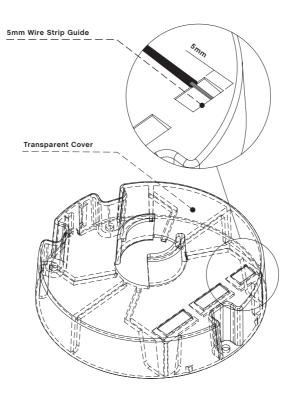
It is advised that any wire exposed with just a single basic layer of insulation is covered with the protective heat shrink provided. (Two sleeves for the basic insulated wire and one sleeve for covering the opening of the pendant cable).
