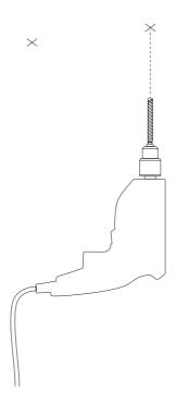
Trim the cable to the desired length, leave 35mm of basic single insulation exposed for wiring.
