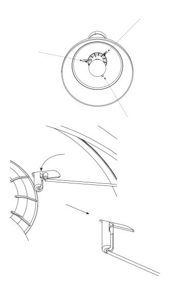
Once the diffuser supports are securely in place, the diffuser can be installed. Place the diffuser into the shade and then gently hook the diffuser supports into the corresponding holes on the reverse side of the diffuser, as shown below.
