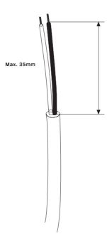
There is a 5mm wire strip guide provided on the internal transparent cover, as shown below. Strip 5mm of exposed wire carefully, ensuring both layers of insulation are intact and not damaged.
