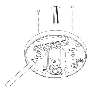
Drill holes and insert wall plugs. Ensure you use the correct type of wall plug for the material you are drilling into.
