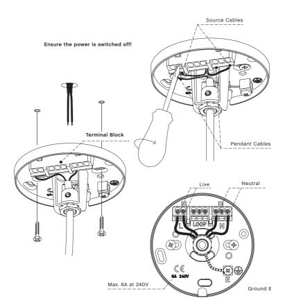
The terminal blocks of the clear ceiling bracket are integrated into a junction box with a loopin feature. This can be utilised in a number of different ways to optimise the wiring of electrical
