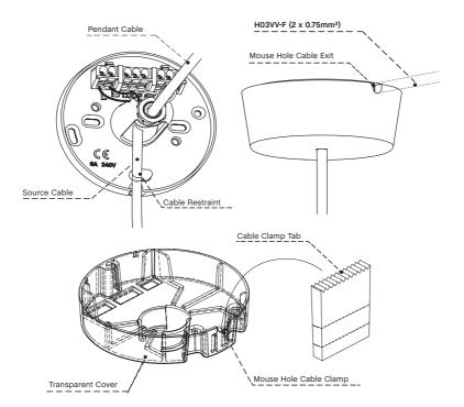
Replace the protective transparent cover over the terminal and clear ceiling bracket, screwing it in place with the three fixings provided. This will isolate the internal electrics during use. Replace the outer magnetic ceiling cap over the assembly, ensuring the mouse hole exits are lined up with the bracket and cap if you inted to utilise this feature.
