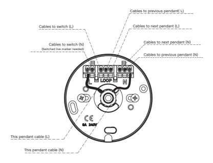
Check to ensure that the protective heat shrink, the cable restraints and cord grip sleeve are still in place after fitting all wires. Check that all of the Live, Neutral and Ground connections are securely connected before switching the power back on at the mains. Ensure there are no loose cables, exposed bare wires and that the clear ceiling bracket is securely fixed to the ceiling.
