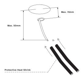
A heat gun can be used to shrink and fix this protective insulation in place, as shown below.
