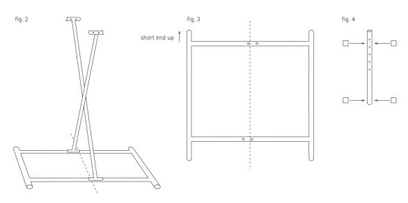
3. Screw together the second side frame on top to the cross brace. Use the enclosed black plastic plug (below) with the base of uprights or self-levelling feet set for uneven floors. For the top of the frame use also plastic, or better rubber-stoppers. However, normally you use the height adjustment rods (also with plastic or rubber stoppers). Never use the rubber stoppers for the base.
