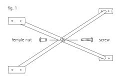
2. Put one frame, with the punched deepenings downward, on the floor or on a table and put the cross braces on the side frame so that the hole of the cross align over the hole of the side frame. (fig. 2). If it doesn't fit, please turn over the cross 180 °.
