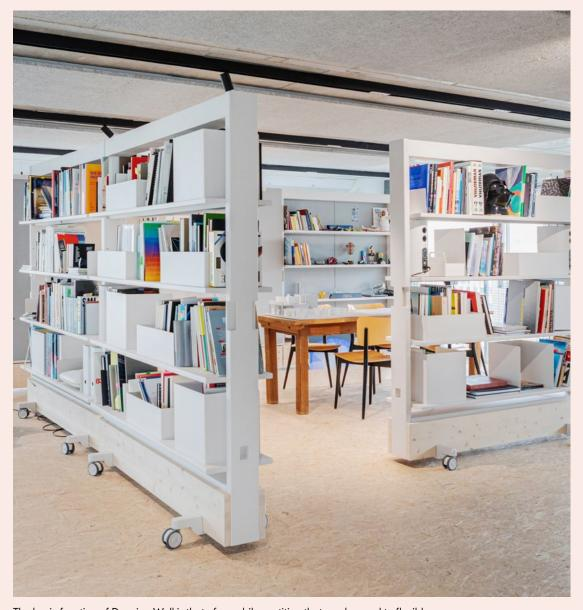
The basic function of Dancing Wall is that of a mobile partition that can be used to flexibly divide offices into zones, while providing vertical work space. It consists of a metal frame, which can be equipped in various configurations: as a bookshelf, TV unit, cloakroom, plant wall, or as a room divider with removable whiteboards and pinboards.
