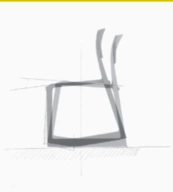
TIP TON, EDWARD BARBER & JAY OSGERBY, 2011 Tip Ton defines a whole new chair typology: the solid plastic chair with forward-tilt action.
